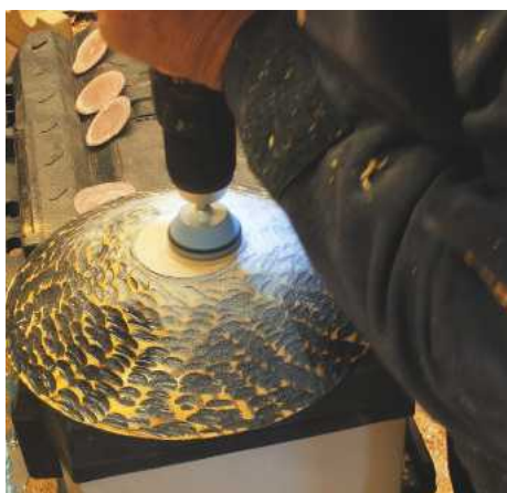
▲ Pic.34 Power sand the base using an arbor mounted in a power drill. Progress through the grits to 400. Finish the bowl with either lemon or Danish oil
